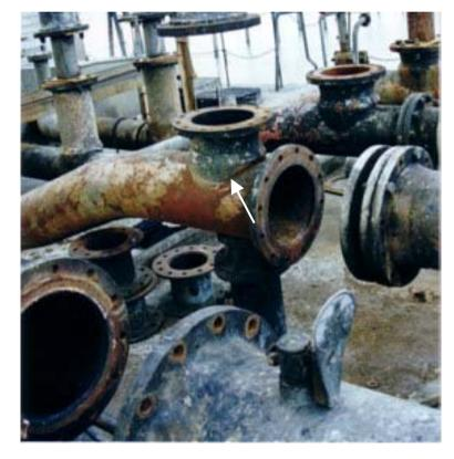
*Fig. 4. Nozzle remote from explosion, note crack propagating from weld, investigated as possible source of air ingress*
