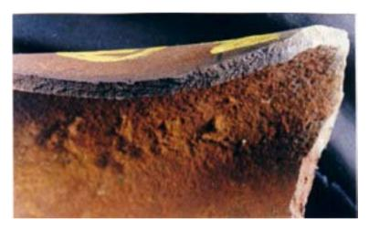
*Fig. 6. Fracture Face with Chevrons indicating origin of fracture and direction of travel.*
