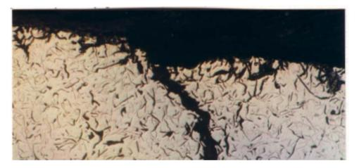
*Fig. 10 Microstructure at 75X showing corrosion, along Graphite flakes and intergranular cracking.*
