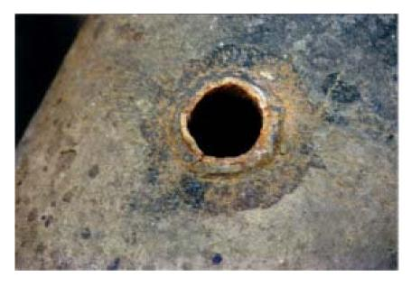
Fig. 3. Weld on main Line, residue beneath 1.5" valve, note cracking in the weld and Luder lines around weld indicating stress field. This was removed for metallographic investigation.
