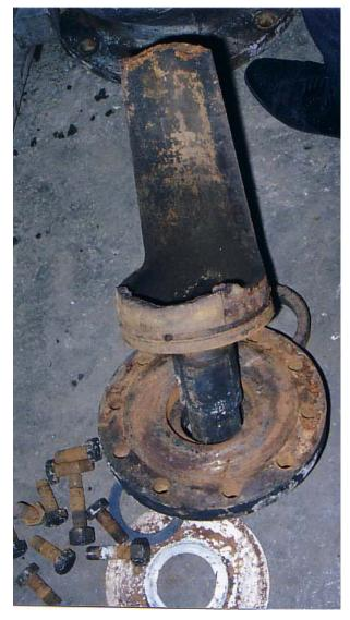
Fig. 9 Fractured plug with downstream side missing
