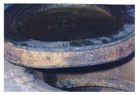
*Fig. 5. Fracture on seat ring of isolating spade, investigated as possible origin of air ingress*
