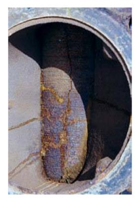
Fig. 7 Cracking in upstream side of plug valve this valve was located above an exploded region of the pipeline this plug valve, large pieces of the plug were found to be missing. In the explosion, the pig trap door was blown off and was not recovered and it is probable that the parts of the plug were also blow out of this door.
