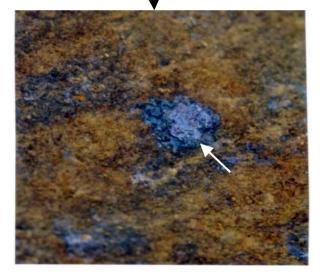
Fig. 12 View under microscope of exploded section of pipe, note melting of oxide layer. Indicative of initiation point of explosion.
