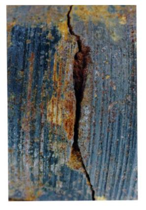
As part of the investigation, valves were removed for examination. It was noted that the plug of one valve was cracked, see Fig.7. This was located on the upstream of the valve, which was positioned on the unused line above the explosion damage seen in Fig. 11. On the downstream side of the cast iron material of construction had suffered corrosion and this had resulted in intergranular cracking. It was therefore apparent that the fracture here had been present prior to the explosion.
