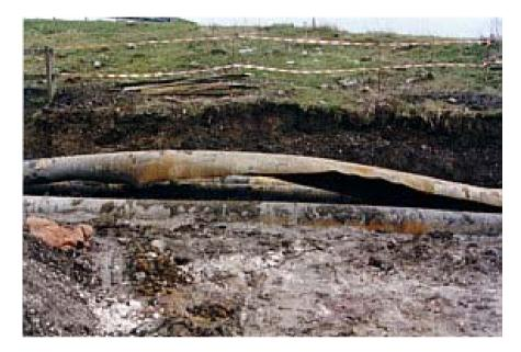
Fig. 2. Side view of exploded pipe.
